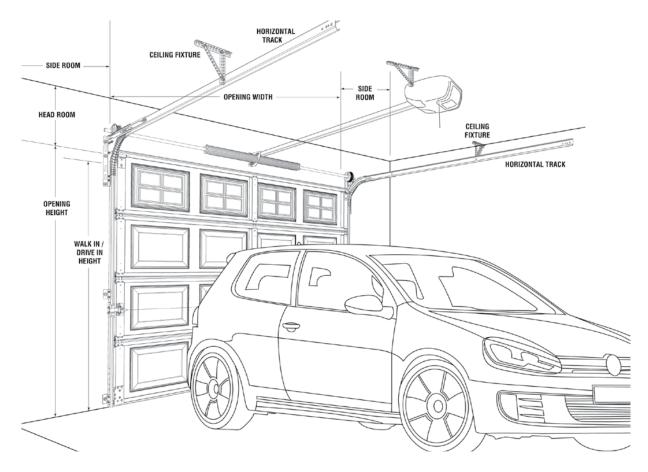
Sectional garage door offers the greatest degree of aesthetic adaptability. It comprises a number of large sections or panels that come in a wide rage of designs and colours. Sectional Garage Doors are most commonly made from pressed steel, but can be manufactured from timber to provide a more natural look.
