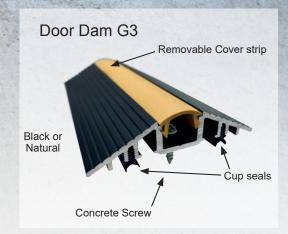
Cleverseal Door Dam G3 Threshold Seal provides a tight, long lasting barrier to prevent water pooling inside your garage. The ground-breaking design of Cleverseal Door Dam G3 is made of hard-wearing aluminium with the additional protection of two bottom PVC cup seals, that compress against the garage floor to provide an immediate tight seal to stop water soaking your garage floor.
